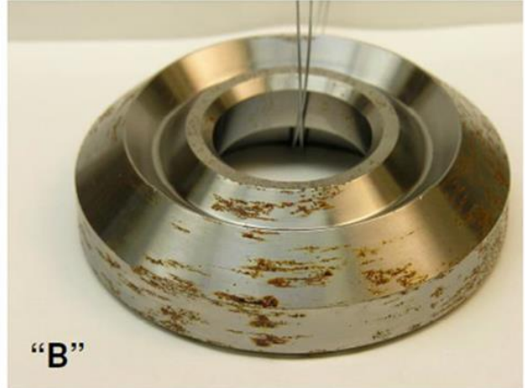
Part #1, coated with Blaser coolant and tested as received, after 24 hours ("A") and 15 days ("B").
